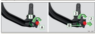
Fig. 148 Lock unlock / pull out hand wheel and turn
