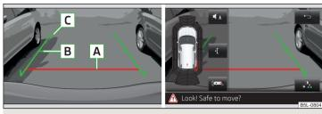
Fig. 140 Infotainment display: Orientation lines / function keys
