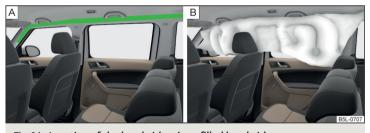
Fig. 14 Location of the head airbag/gas-filled head airbag
