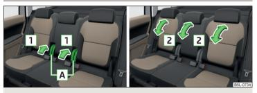
Fig. 68 Adjusting the seat backrest
