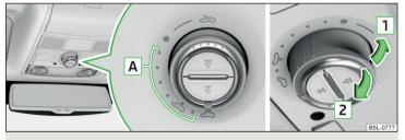
Fig. 43 Operation of the sliding/tilting roof
