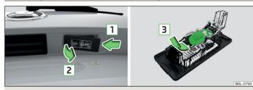
Fig. 203 Remove the number plate light/replace the bulb
