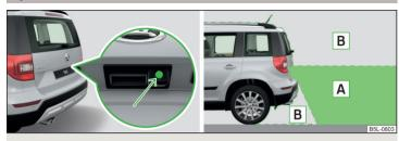
Fig. 139 Position of the camera / monitored area
