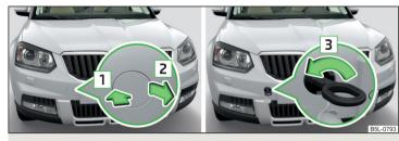
Fig. 182 Removing the cap / fitting the towing eye
