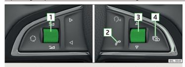
$Fig.\,118\quad \textbf{Multifunction steering wheel: Control buttons for the telephone}$
