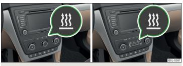
Fig. 114 Button for switching on/off the system directly on the operating part of the air conditioning/Climatronic
