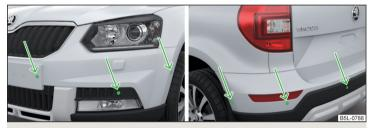
Fig. 137 Location of the ultrasonic sensors: front / rear
