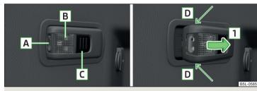
Fig. 104 Light operation / removal
