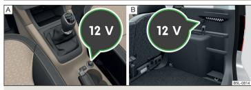
Fig. 83 12-Volt power outlet in the front centre console / in the boot
