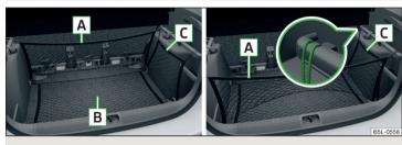
Fig. 96 Fastening examples for nets
