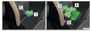
Fig. 79 Open cup holder in the central console / adjust holder size
