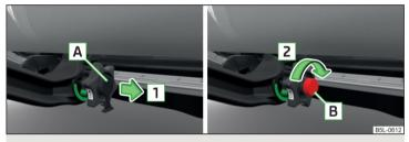
Fig. 153 Removing the lock cover/releasing the lock
