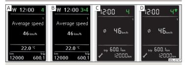
Fig. 29 Information on the selected gear / Gear recommendation
