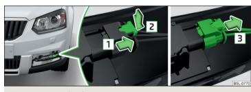
Fig. 201 Remove the plug
