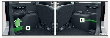
Fig. 102 Storage compartment on the left / right
