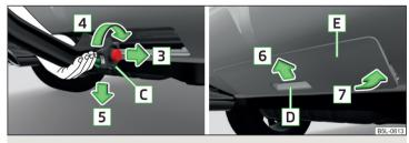
Fig. 154 Removing the two bar/placing the cover on the rear bumper
