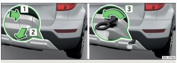
Fig. 183 Removing the cap / fitting the towing eye
