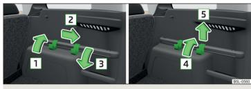
Fig. 98 Sliding hook on the mounting bar / removing hook
