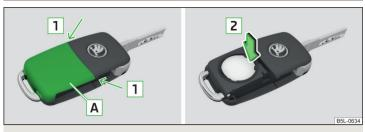
Fig. 184 Remove cover/take out battery
