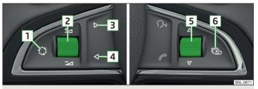
Fig. 120 Multifunction steering wheel: control buttons
