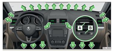
Fig. 109 Air vents at the front
