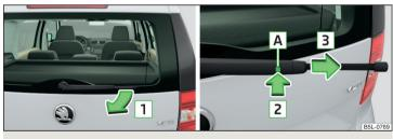
Fig. 192 Rear window wiper blade
