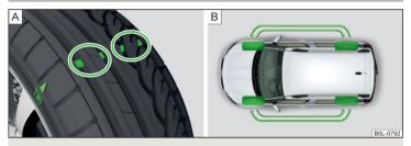
Fig. 167 Principle sketch: Replace tyre tread with wear indicators / wheels
