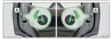
Fig. 188 Emergency locking: Left/right rear door
