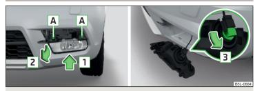
Fig. 202 Principle sketch: Remove the number plate light / replace the bulb
