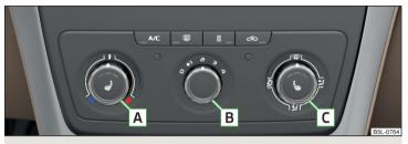
Fig. 112 Controls of the air conditioning
