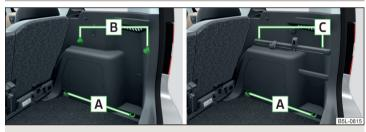
Fig. 95 Fasteners: Version 1/version 2
