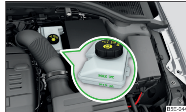
Fig. 189 Brake fluid reservoir
