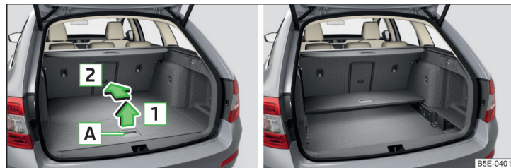
Fig. 115 Fold up variable loading floor / folded variable cargo floor in the upper position
