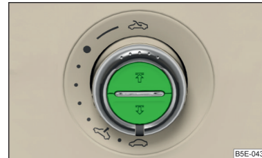
Fig. 49 Operation of the sun blinds
