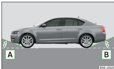
Fig. 238 Principle sketch: Departure angle
