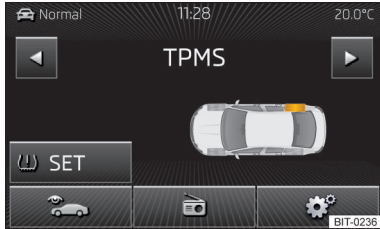
Fig. 164 Button for storing the pressure values /example of the display: the system is indicating a change in tyre pressure in the rear right-hand tyre
