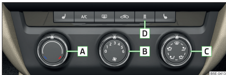
Fig. 125 Controls of the air conditioning
