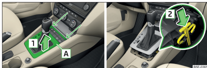
Fig. 216 Selector lever-emergency unlocking
