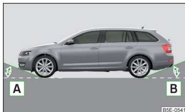
Fig. 239 Schematic diagram: Departure angle
