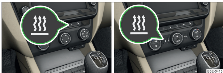
Fig. 127 Button for switching on/off the system directly on the operating part of the air conditioning/Climatronic
