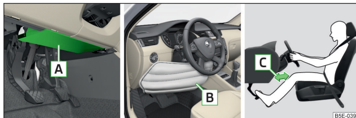
Fig. 10 Installation of the airbag / Gas-filled Airbag / Safe distance between the legs and the instrument panel
