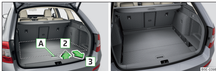
Fig. 114 Set variable loading floor to the lower position / variable loading floor in the lower position
