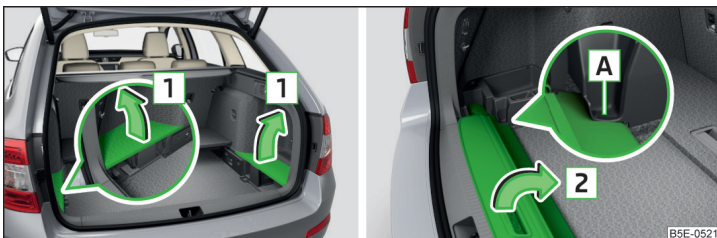
Fig. 108 Remove the side panels of the luggage compartment/stow the roll-up luggage compartment cover
