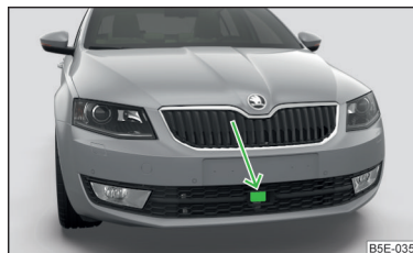
Fig. 148 Mounting location of the radar sensor
