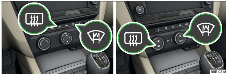
Fig. 60 Buttons for the front and rear window heater: manual air conditioning, heating/Climatronic
