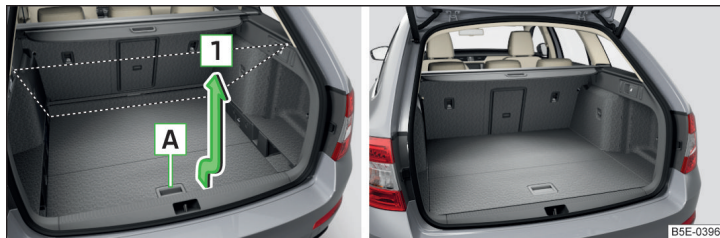
Fig. 113 Set variable loading floor to the upper position / variable loading floor in the upper position
