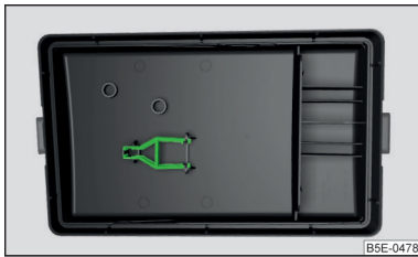
Fig. 223 Cover for the fuse box in the engine compartment: Plastic clip for fuses
