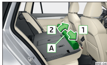
Fig. 119 Removing the net partition housing
