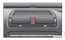
Fig. 37 Dash panel: Switch for hazard warning lights
