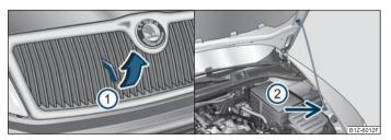
Fig. 121 Radiator grille: Release lever / securing the bonnet with the bonnet support
