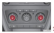
Fig. 54 Dash panel: Regulator for front seat heating
