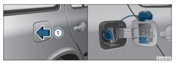
Fig. 119 Right rear side of the vehicle: Open fuel filler flap/fuel filler flap with cap unscrewed
