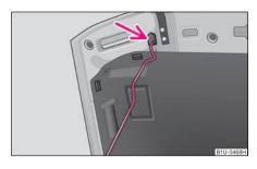
Fig. 16 Securing the bonnet with the bonnet support
