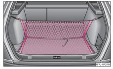
Fig. 67 Fixing net: double horizontal pocket, floor fixing net
