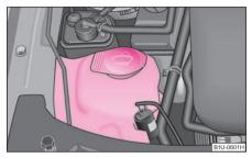
Fig. 152 Engine compartment: Windshield washer fluid reservoir
