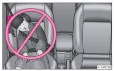
Fig. 126 Seated position of an unprotected child at risk from side airbag
