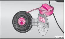
Fig. 141 Fuel filler flap with cap unscrewed
