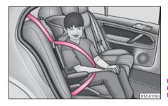
Fig. 130 Child seat in Group 2 installed on the rear seat facing the direction of travel
