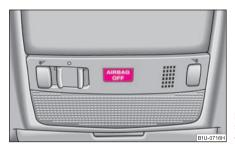
Fig. 124 Indicator light for a switched off front seat passenger airbag
