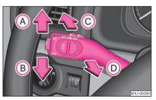
Fig. 9 Turn signal and main beam lever
