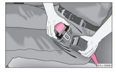
Fig. 115 Fasten pelvic belt
