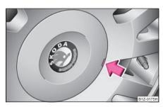
Fig. 162 Pulling off wheel trim cap on light alloy wheels
