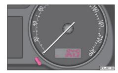
Fig. 19 Instrument cluster: Counter for distance driven
