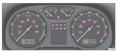
Fig. 26 Instrument cluster with warning lights
