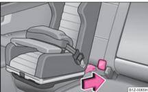
Fig. 133 The ISOFIX child seat is pushed into the mounting funnels
