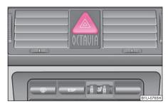
Fig. 44 Dash panel: Switch for hazard warning lights
