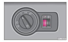
Fig. 42 Dash panel: Instrument lighting
