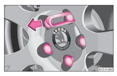
Fig. 161 Removing the cap.
