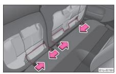
Fig. 62 Removing seat cushions
