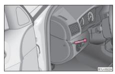
Fig. 169 Fuse cover: left side of the dash panel
