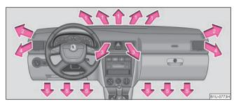
Fig. 94 Air outlet vents
