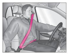
Fig. 111 Routing of webbing over the shoulders and the lap belt
