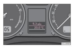
Fig. 23 Instrument cluster: small information display
