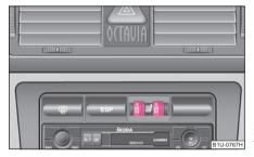
Fig. 63 Dash panel: Control dial for heating the front seats
