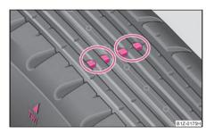
Fig. 154 Tyre tread with wear indicators
