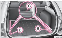
Fig. 74 Luggage compartment: Remove carrier rails
