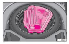
Fig. 157 Luggage compartment: storage compartment for vehicle tool kit
