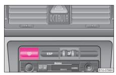
Fig. 48 Switch for rear window heater
