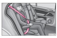
Fig. 131 Child seat in Group 3 installed on the rear seat facing the direction of travel
