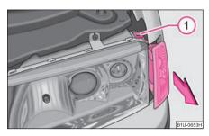
Fig. 178 Removing the light bulb for the turn signal light
