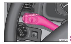
Fig. 45 Turn signal and main beam lever
