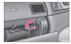
Fig. 123 Storage compartment: Switch for the front passenger airbag(s)
