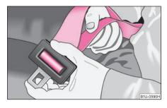
Fig. 116 Extending the pelvic belt
