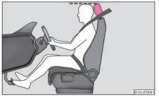
Fig. 107 The correct head restraint adjustment for the driver
