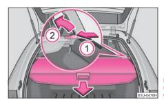
Fig. 72 Luggage compartment: removing the foldable luggage compartment cover
