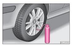
Fig. 158 Vehicle tool kit: Spray for repairing a tyre
