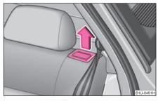
Fig. 60 Unlock the seat backrest
