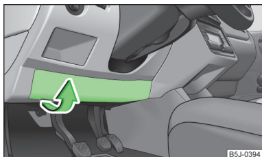
Fig. 157 Underside of the dash panel: Distribution board cover.
