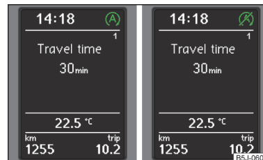
Fig. 120 Maxi DOT display: Engine is automatically switched off / automatic engine cut off is not possible
