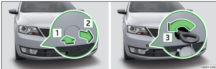
Fig. 141 Removing the cap/installing the towing eye
