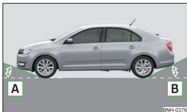
Fig. 164 Principle sketch: Departure angle
