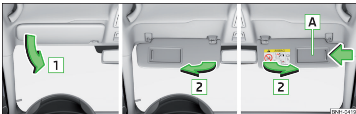
Fig. 47 Fold down the cover / swivel cover to the door and slide the mirror cover
