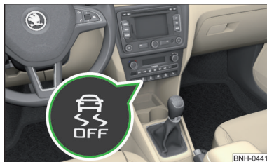
Fig. 97 Press the ESC system: Activating/deactivating TCS
