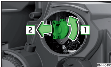
Fig. 155 Replacing the bulb for main beam and separate daytime running lights
