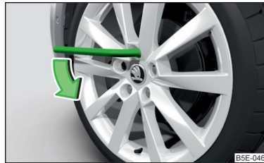
Fig. 133 Changing a wheel: Loosening the wheel bolts
