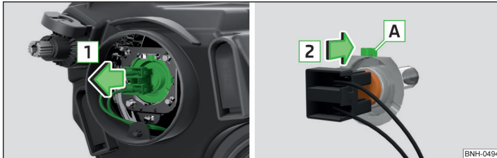
Fig. 154 Changing the bulb for the low beam
