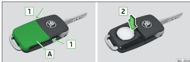
Fig. 143 Remove cover/take out battery
