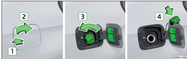
Fig. 116 Open fuel filler flap / unscrew tank cap / place the tank cap on the fuel filler flap
